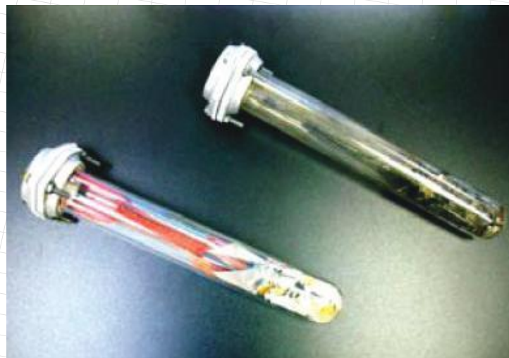
The photo above, courtesy of Eltek Labs, shows one tube prior to aging and another tube after aging.
