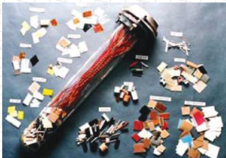
The photo above, courtesy of Eltek Labs, shows a typical Sealed Tube with representative samples of materials prior to testing.
