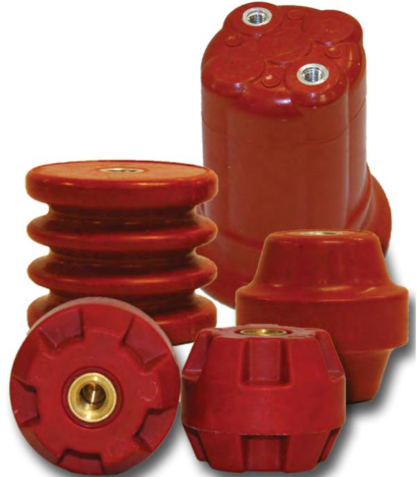
The attachment of the support of bus bars is covered in Annex G Section 3.3. The bolts used to secure the bus bar to a standoff insulator must be 3/8-16 steel or larger and torqued to 20 pound-feet. Standoff insulators that have inserts smaller than 3/8-16 may be used for support of live parts, but the assembly would have to be tested to achieve the high SCCR ratings. Any substitution of those standoffs insulators would likely require a new SCCR test.
