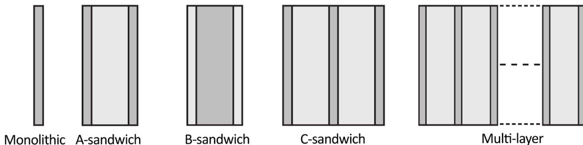
Understanding materials suitable for the application and designing the radome so it optimizes those materials is key, but radome configuration is just as important.
