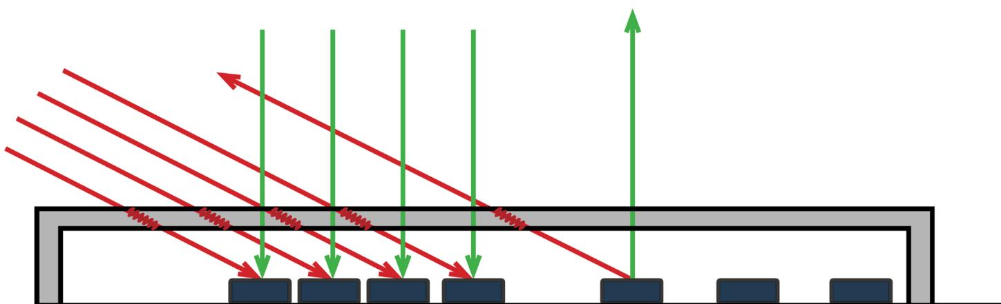
If the goal is to minimize reflection of the incident wave, introducing a surface at the lowest wave amplitude is ideal. This occurs at the half-wavelength point and this logic applies to the radome. Assuming the material selected is proper for the application, the radome thickness and the distance to the antenna should be in multiples of half-wavelengths.
